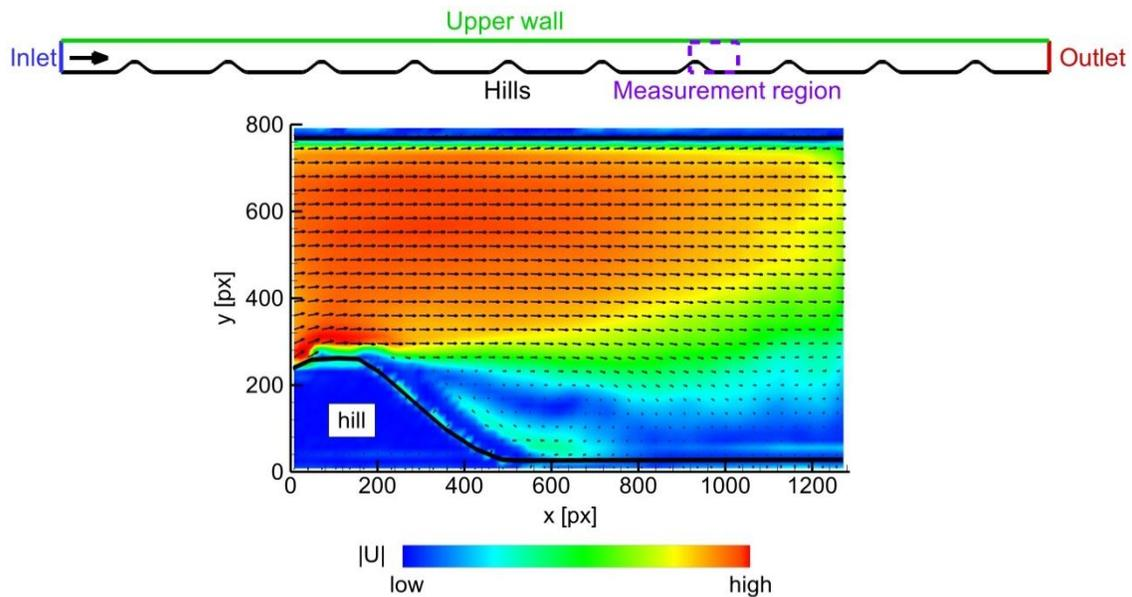
Figure 1: Sketch of the experiment and the mean velocity / displacement field (not every vector shown)
