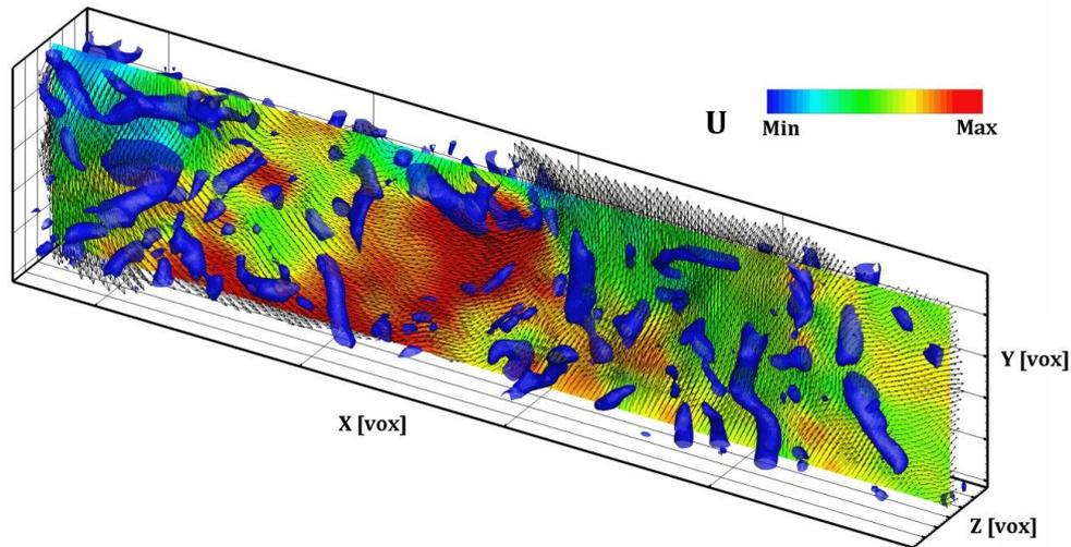
Contour of the U component of the velocity field (arbitrary units) on the XY mid-plane and isosurfaces of the second invariant of the velocity gradient tensor  $Q > 0$ .
