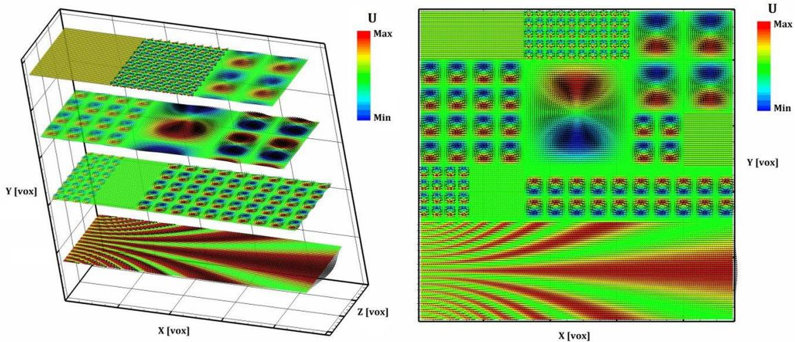
Contour of the  $U$  component (arbitrary units) of the velocity field and vector representation on XZ planes (left) and on the mid-plane (right).
